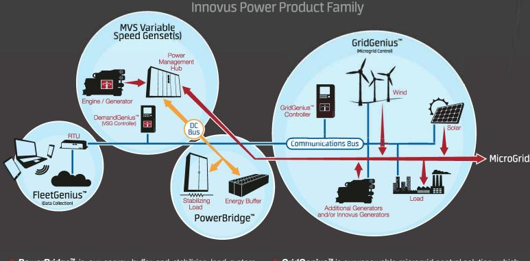
**PowerBridge**<sup>™</sup> is our energy buffer and stabilizing load system which manages overproduction of renewable generation and allows engine off and stabilization of third party fixed speed generators.
